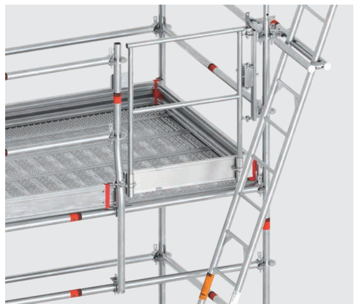
External ladder access with scaffolding ladder, ladder holder and self-closing swing door
