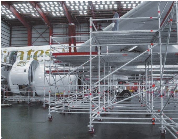
Mobile aircraft maintenance scaffolding
